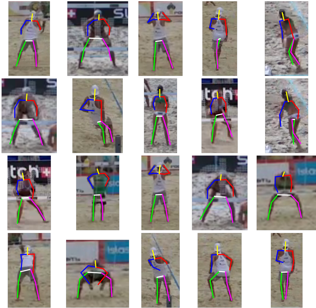
Figure 8: Additional results on Volleyball [1] : Samples of our results using the coarse-to-fine model on 2D human pose estimation are presented.
