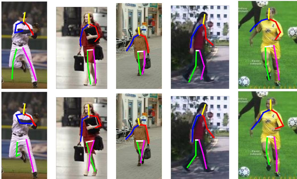
Figure 1: Additional results on model refinement - PARSE: Additional results for the coarse-to-fine model using the cascade of ConvNets are presented from the PARSE dataset [6]. On the top row the result of a single ConvNet is presented, while on the bottom row the refined result using the cascade of ConvNets.
