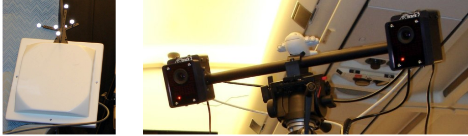
Fig. 7. Antenna with IR-Marker and A.R.T. Tracking System
