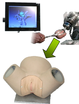
Figure 1. Delivery simulator: Virtual simulator on the screen, phantom head on robot's arm, female body phantom
