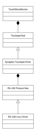
Figure 4.6: Driver layers of raw data provider service
