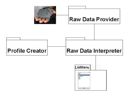
Figure 4.2: Subsystem Decomposition of TouchGlove
