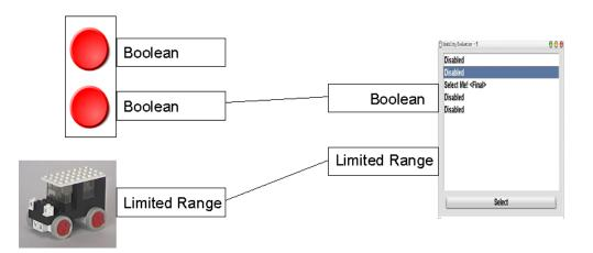
Figure 3.5: Example of intersection matching between a two-button device, a tracked tangible device and a list menu
