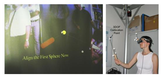
Figure 1.6: HMD calibration with a pointing device
