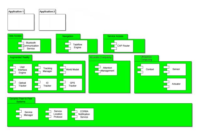
Figure 1.1: A layered architecture for the DWARF framework
