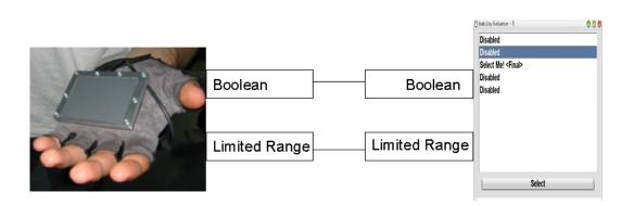
Figure 3.4: Example of subset matching between the TouchGlove and a slider shown in a HMD
