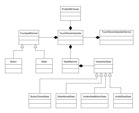
Figure 4.7: Raw Data Interpreter Class Diagram
