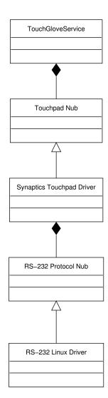
Figure 2.1: Driver layer example for touchpad
