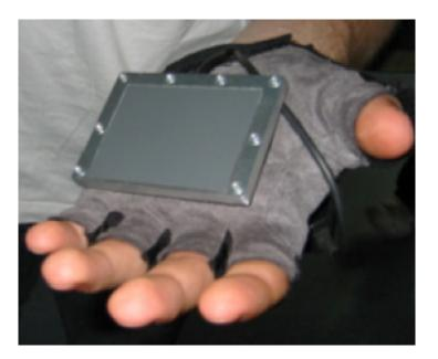
Figure 4.1: The TouchGlove input device
