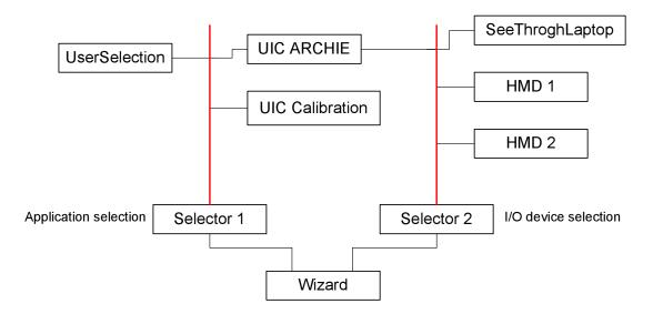
**Figure 9.1:** A concept for the design of a central MenuDisplay component which handles all menus coming from the Selector at once. The user can navigate through the menus and commit them when everthing is configured by him.
