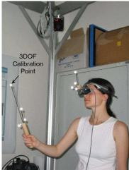
Figure 2.2: HMD calibration with a pointing device
