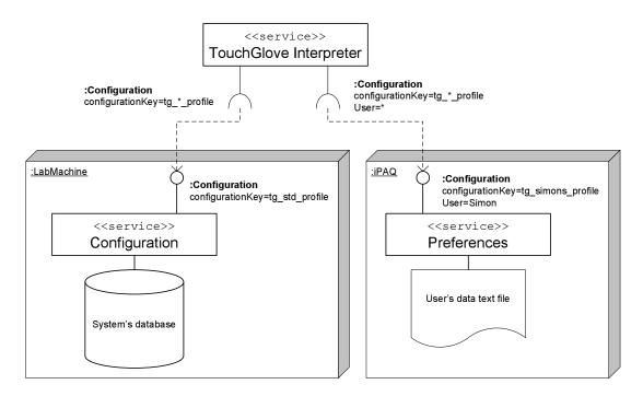
**Figure 4.4:** There are two different sources which provide a suitable profile for the TouchGlove Interpreter service.
