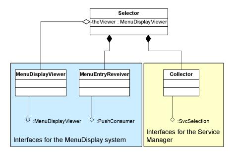
Figure 6.2: The system design of the Selector service
