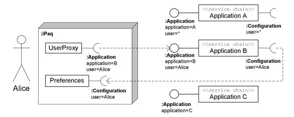
Figure 4.2: Approach: Configuration of DWARF applications by introducing a Configuration need
