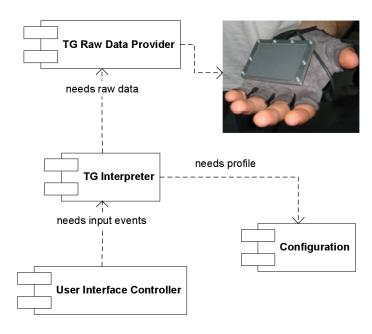
Figure 3.3: The *TouchGlove* subsystem
