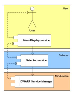
Figure 6.1: The Selector service: bridge between middleware and user
