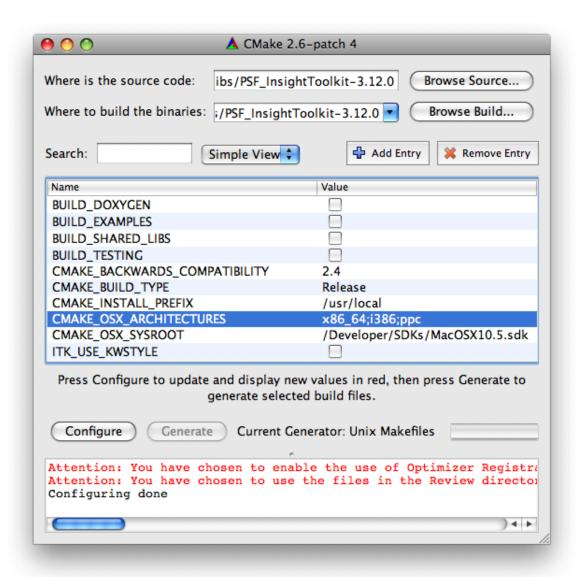
Figure 8: Typical ITK settings that are appropriate for OsiriX plugin development. If you have enabled optimized registration methods and the review code you should also see two warning in the output.
