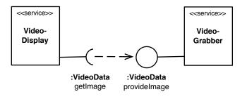
Figure 1.1: Example: Providing a video image
