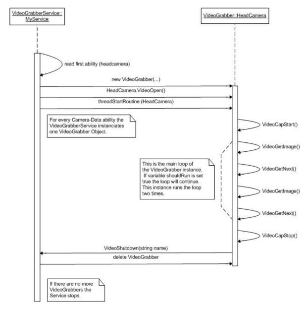
Figure 3.12: VideoGrabber UML Sequence Diagram
