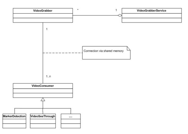
Figure 3.10: VideoGrabber UML Class-Diagram
