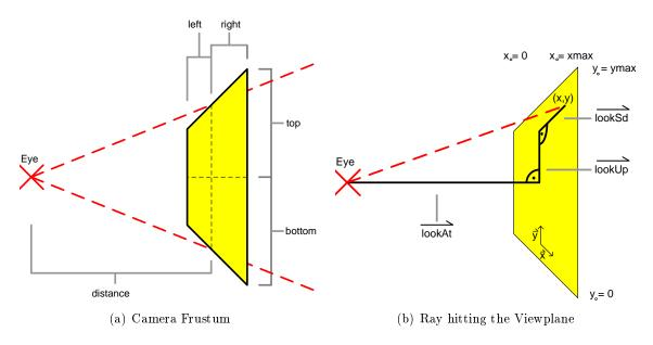
Figure 5.2: Raytracing Camera
