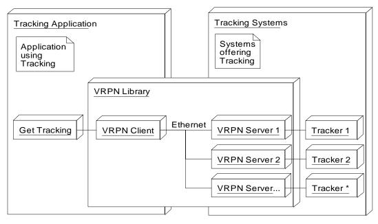
Figure 2.5: VRPN Communication Diagram
