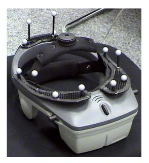
Figure 5.5: Head Mounted Display (HMD) with Infrared Markers
