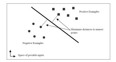
Figure 2.7: An example for a linear support vector machine.
