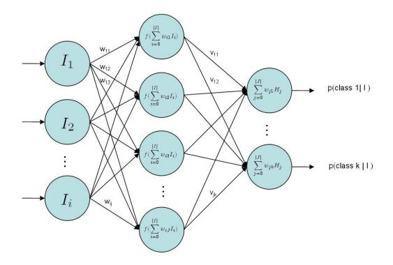
Figure 2.8: A scheme for a feed forward network. The input is the vector I with its entries  $I_1..I_i$  and the length I. The results are the estimated probabilities for the special class. s
