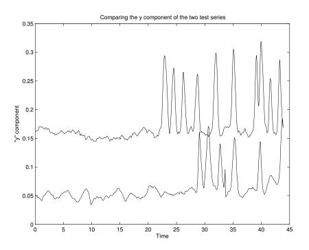
**Figure 7.3:** Comparing the *y* component of the ART and ARToolKit position vectors: Because the two coordinate systems coincidentally pointed to the same direction, the *y* component must show related behavior. The ARToolKit values (lower line) shows an offset of several seconds compared with the ART target (top line).
