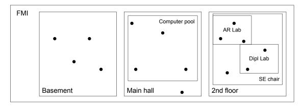
**Figure 4.3:** Example of a spatial index of the FMI building: The rectangles show the partition of the Spatial Relationship Graph nodes (black dots). The classification are physical characteristics of the building itself, i.e. main halls, floors, rooms.
