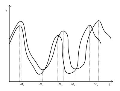
Figure 6.2: Comparing the time distance between the extrema of the speed plot
