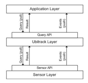
Figure 1.6: The three layer Ubitrack architecture model
