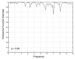
**Figure 7.11:** Coherence function of the angular velocity
