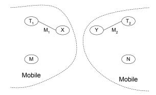
**Figure 4.10:** The real constructed Spatial Relationship Graph containing anonymous objects X and Y: The actual measurements  $M_i$  are not between the sensors  $T_i$  and the real locatables M and N, but between the sensors and the anonymous objects X and Y.
