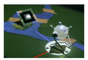
**Figure 2.8:** Picture of an example scenario implemented in DWARF: An AR Toolkit marker is tracked by a mobile camera which is attached to an ART target. A virtual sheep is projected onto the AR Toolkit marker relative to the ART coordinate system.
