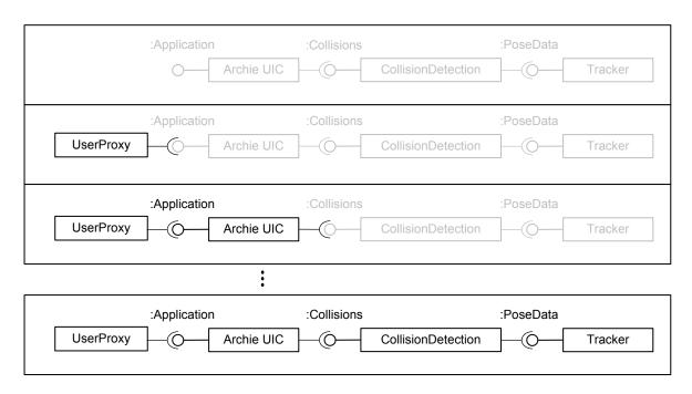
**Figure 3.1:** With the start of the UserProxy service a whole service chain is started on demand. This is a simple example of booting whole DWARF applications. Further information can be found in [53].
