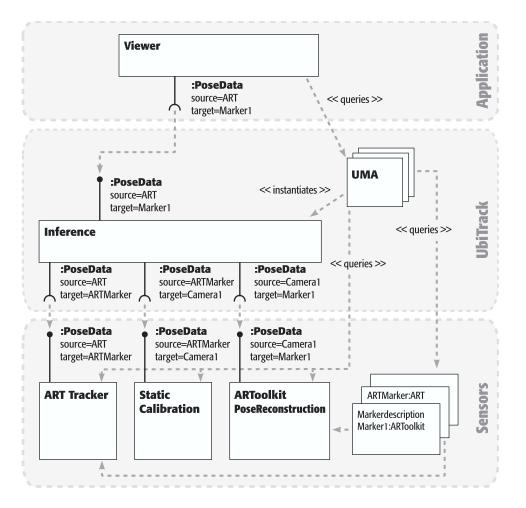
Figure 2.12: The example scenario modeled by DWARF services (which are data flow components)
