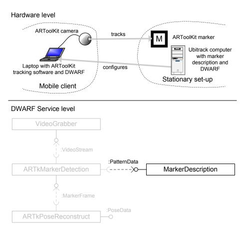
**Figure 3.2:** Simple bootstrapping example for a tracking network based on DWARF. When the MarkerDescription is started, the DWARF Service Manager starts the ARTkMarkerDetection including all depending services. Therefore if the marker description is available, a new PoseData ability is generated.
