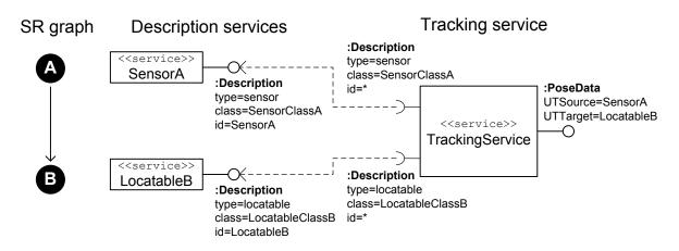
**Figure 5.2:** Sensor and locatable description are merged in the tracking service. The PoseData ability corresponds to the given configuration, i.e. UTSource and UTTarget are set to the values from the description services.
