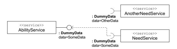
**Figure 2.5:** This UML diagram shows an example session of three services. Two of them are connected, one is not since the predicate does not match. The annotations in the figure describe the individual UML notations.
