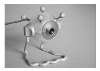
Figure 9.3: iBot camera with attached ART target
