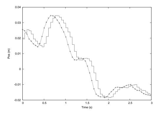
Figure 9.5: ART measurements without prediction shifted by 100ms.
