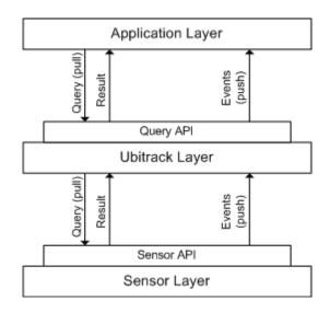
Figure 1.1: The three layer Ubitrack architecture model
