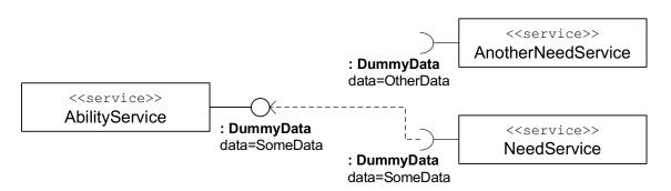
Figure 2.5: This UML diagram shows an example session of three services. Two of them are connected, one is not since the predicate did not match. The annotations in the figure describe the individual UML notations.
