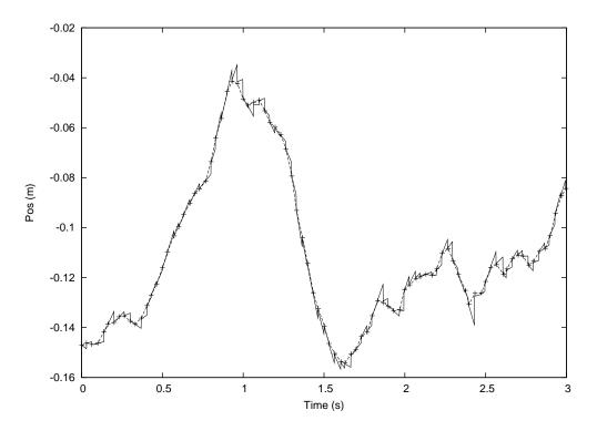
Figure 9.12: AR Toolkit measurements predicted using a kalman filter.
