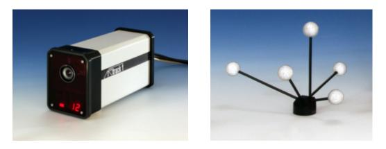
Figure 9.1: ART camera and a typical target
