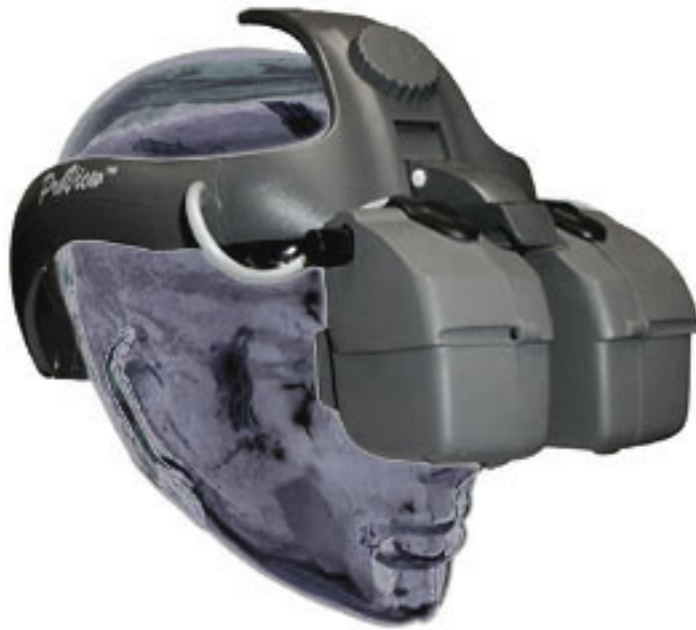
Abbildung 1.3: ProView XL50 Video See-Through Head-Mounted Display
