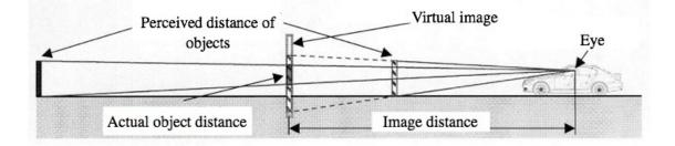
Figure 3.6: Conformal visualization (Courtesy of [4])
