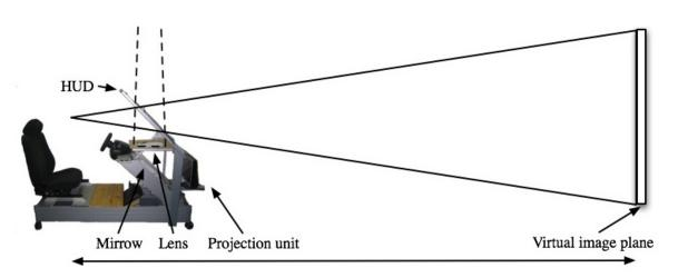
Figure 5.4: Optical setup
