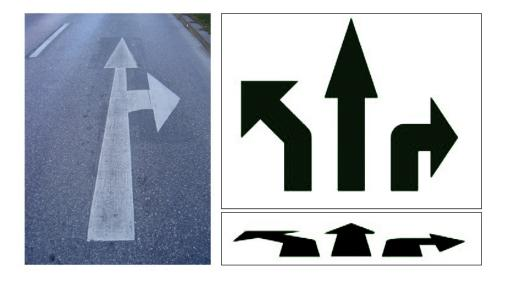
Figure 4.5: Left:Lane marking; Right top:Bird's eye view, Right below:Perspective view
