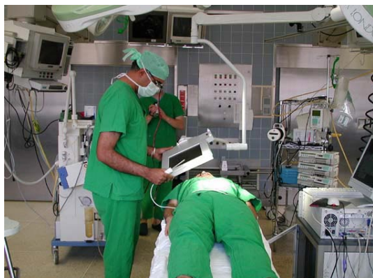
(a) The hardware setup of the MEDARPA system using the swivel arm in a real operating theater environment. The surgeon is holding an Endo-stabilizer.
