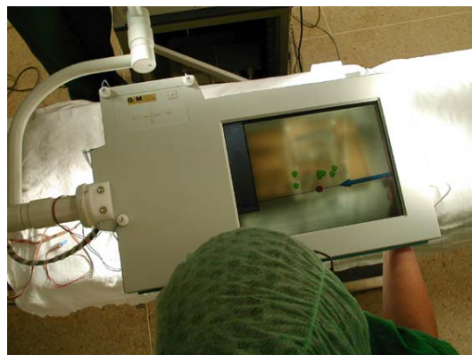
(b) The AR-window is a semitransparent combiner plate. This enables the projection of virtual objects on top of the real world view. While looking through this window, the ports can be planned intra-operatively, wherefore the Endo-stabilizer's axis (blue) must intersect the region of interest (red).
