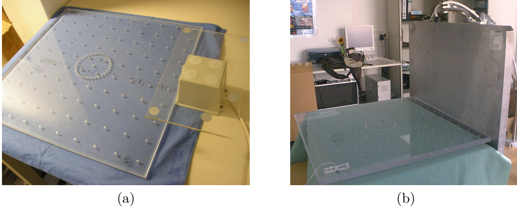
Figure 6.2: The experimental setup for the plate experiments with the mid-range transmitter (a) and flat transmitter (b). The operating volume was totally free of distortion causing materials like metallic objects or electrical devices.
