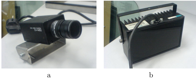
Figure 3.2: SiViT Components: a) IR Camera Pentax CV-M50 , b) IR-LED Spotlight
