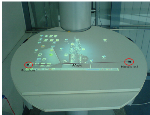
Figure 6.2: Microphone placement on the table
