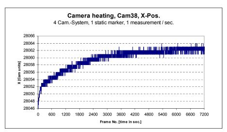
Figure 2.5: Strong effects of heat development in a camera
