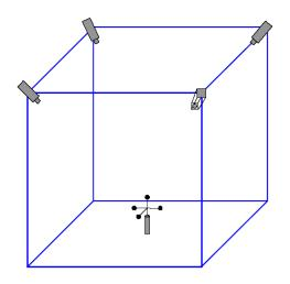
Figure 1.6: A typical A.R.T. setup with four cameras
