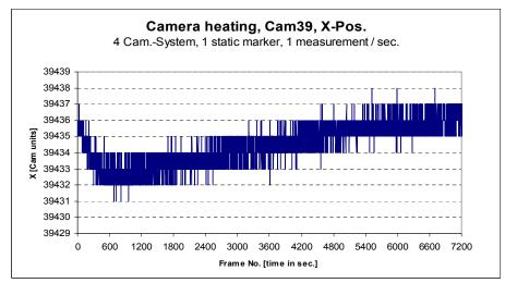
Figure 2.6: Weak effects of heat development in a camera
