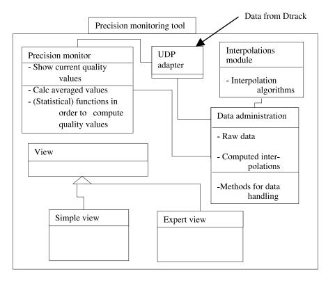
Figure 3.2: The architecture of the monitoring tool
