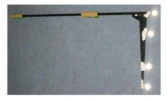
Figure A.3: A bar for scanning the tracking area fast and efficiently
