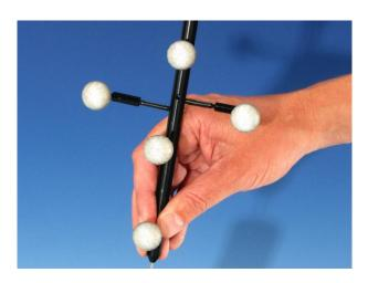
Figure 1.5: Marker from A.R.T. forming a body
