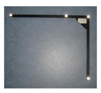
Figure 2.1: The A.R.T. calibration angle
