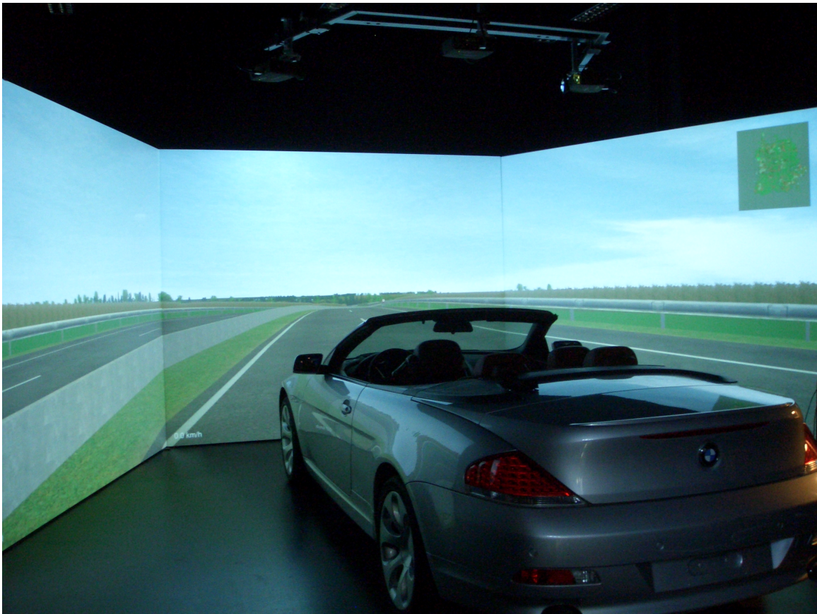
Figure 6: Driving simulator at LfE, TUM
