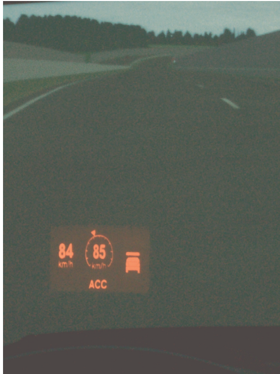
Figure 2: 2D optical information – current speed, wanted speed and desired following distance shown in HUD
