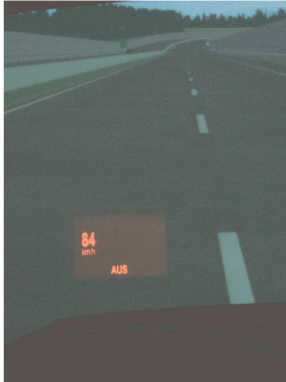
Figure 1: Concept "Aus" – only current speed is shown in HUD
