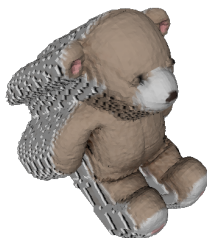
Figure 3.7.: Formation of view-dependent protrusions in the generation of single-frame SDFs
