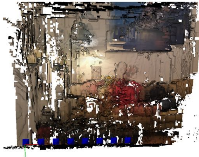
Figure 5.12: Reconstruction of non-rigid scene without deforming already obtained depth information appropriately: Subsequent point clouds are simply integrated into the TSDF without accounting for non-rigidity.
