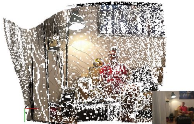
Figure 5.9: Reconstruction after marching cubes of the TSDF with two integrated point clouds: Original input image is shown at the bottom.
