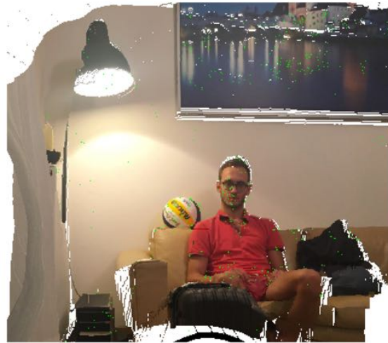
Figure 5.8: Reprojection of fully dense disparity map and triangulated feature points (green): The scene projected is highly detailed and depth continuities are preserved.
