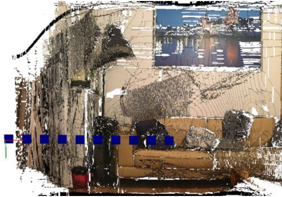
Figure 5.11: Reconstruction of rigid scene with perfect camera poses and noise: As the marching cubes weight has been set to minimum, also voxels filled only once with noise are considered for reconstruction.
