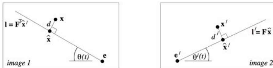
Figure 4.17: Minimization of the reprojection error in 2D: Since solving the reprojection in 3D is not suitable, the perpendicular distance between the estimated epipolar lines and the noisy point correspondences can be minimized in 2D; Adopted from [53].
