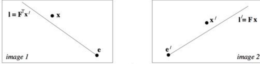
Figure 4.15: Violation of the epipolar constraint in 2D: As a result from noisy image acquisition \mathbf{x} and \mathbf{x}' do not satisfy the epipolar constraint, thus they do not lie on the corresponding epipolar line; Adopted from [53].
