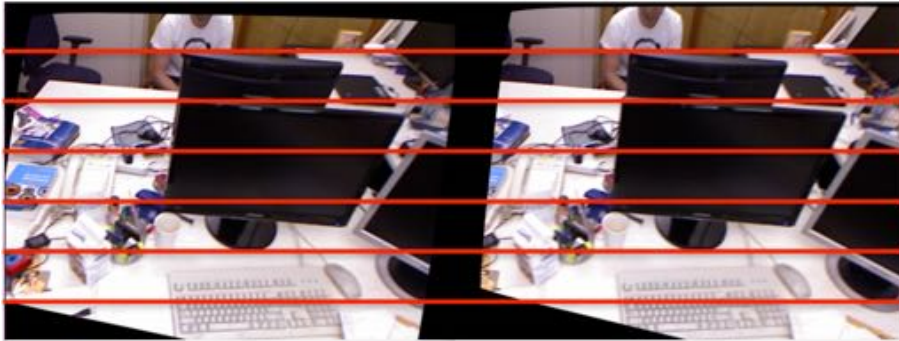
Figure 4.10: Example of epipolar lines after rectification for the uncalibrated case: From the input Figure 4.6, now the epipolar lines are horizontally aligned; Point correspondences only differ in x-direction as indicated by the red lines; TUM RGB-D dataset: [130]
