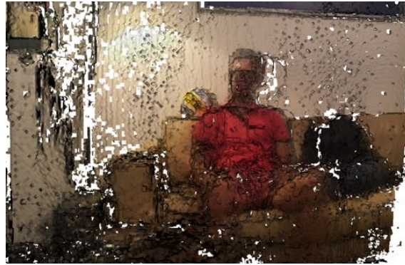
Figure 5.13: Reconstruction of non-rigid scene without appropriate deformation: Another example of bad reconstruction results without incorporation of non-rigid transformations.
