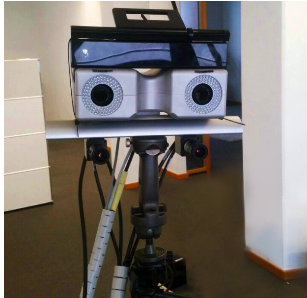
Figure 3.5: Framos OTS camera mounted between Microsoft Kinect v2 and two RGB cameras.
