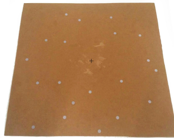
Figure 3.6: The cardboard plane with 20 retro reflective markers attached to it
