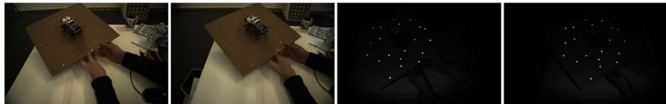
Color stereo views for video sequence and monochrome stereo for marker detection and pose estimation
