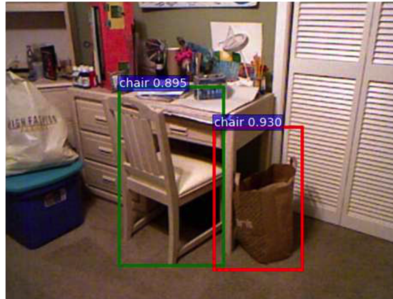
Fig. 1: RGB images could provide ambiguities which lead to a failure: the detection in the red box is the result of RBD object detection.
